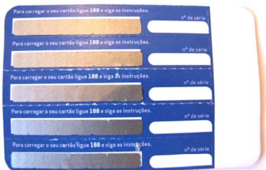
A 'new' card created by successful blade attack
