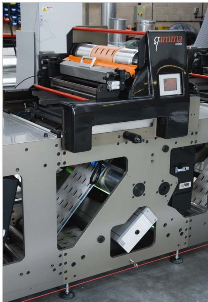
Manufacturers of airtime reload cards often utilise specialist equipment such as the Edale Gamma press (above)
