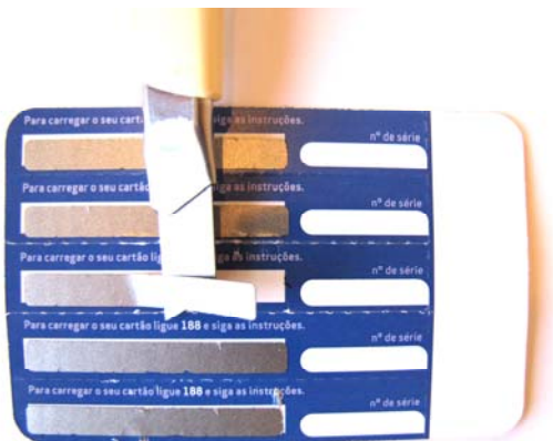
Images show how insecure cards can be 'breached' with a sharp blade, the codes viewed and then the labels replaced
