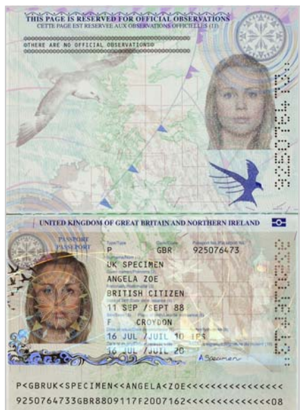
The movement of the chip to within the cover and the addition of an additional bearer photograph should prevent substitution attacks. Note the pinhole numbering
