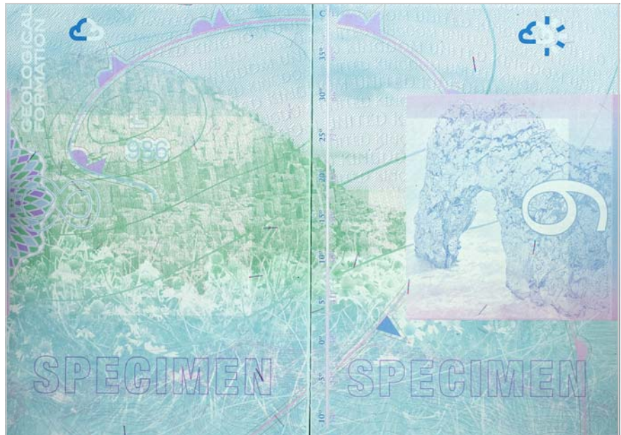
Close register between visa page sections and the use of multicoloured security fibres in the paper along with weather symbols and complex background security offer complex protection
